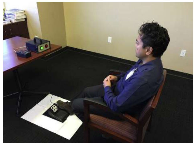
Fig 2. Using the RT-2S Reaction Time tester, subjects were seated with pedals fixed at a distance that corresponded to the patient's usual driving position, allowing for a comfortable application of their right foot to the gas or brake pedal.
