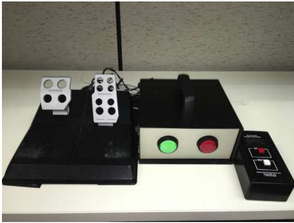
Fig 1. Brake reaction time was measured using an RT-2S Reaction Time tester (Advanced Therapy Products, Glen Allen, VA).
